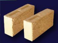
100mm Split Face Block 390mm x 90mm x 190mm One core is solid in every three blocks for splitting corners Code 10-121
